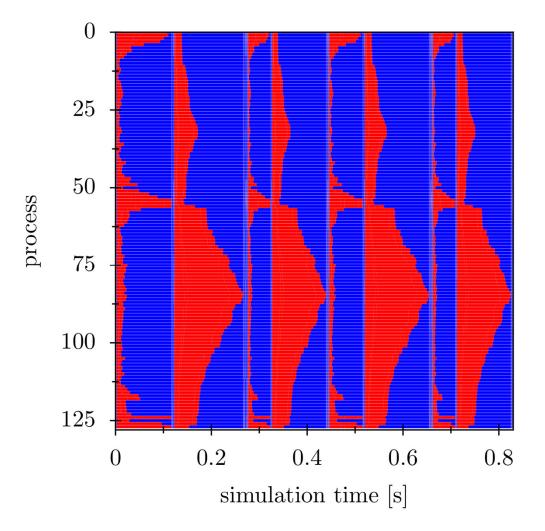
Computational phase diagram from the MPI based GADGET code (used for Nbody and SPH simulations) using 1M particles over four time steps on 128 procs.
